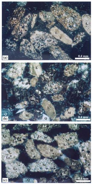
Fig. 4 Particles of fine aggregates. (a) Sample T1, (b) Sample T5, and (c) Sample T7. L = limestone, Ls = Siliceous limestone, M = Marble, Q = Quartz, G = Gneiss, So = Carbonaceous schist, Sc = Calc schist.
