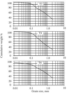
Fig. 2 Grain size distribution curves of fine aggregates.
