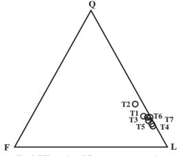
Fig. 3 QFL modes of fine aggregate samples.
