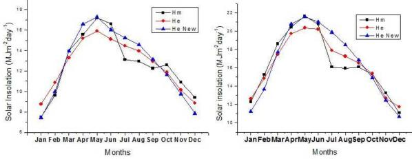
Figure 1: (a) Variation of radiation with months for Biratnagar (b) Variation of radiation with months for Kathmandu
