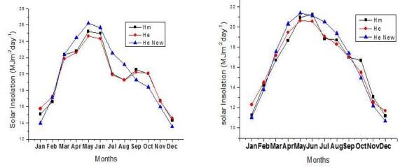
Figure 1: (c) Variation of radiation with months for Pokhara (d) Variation of radiation with months for Junla
