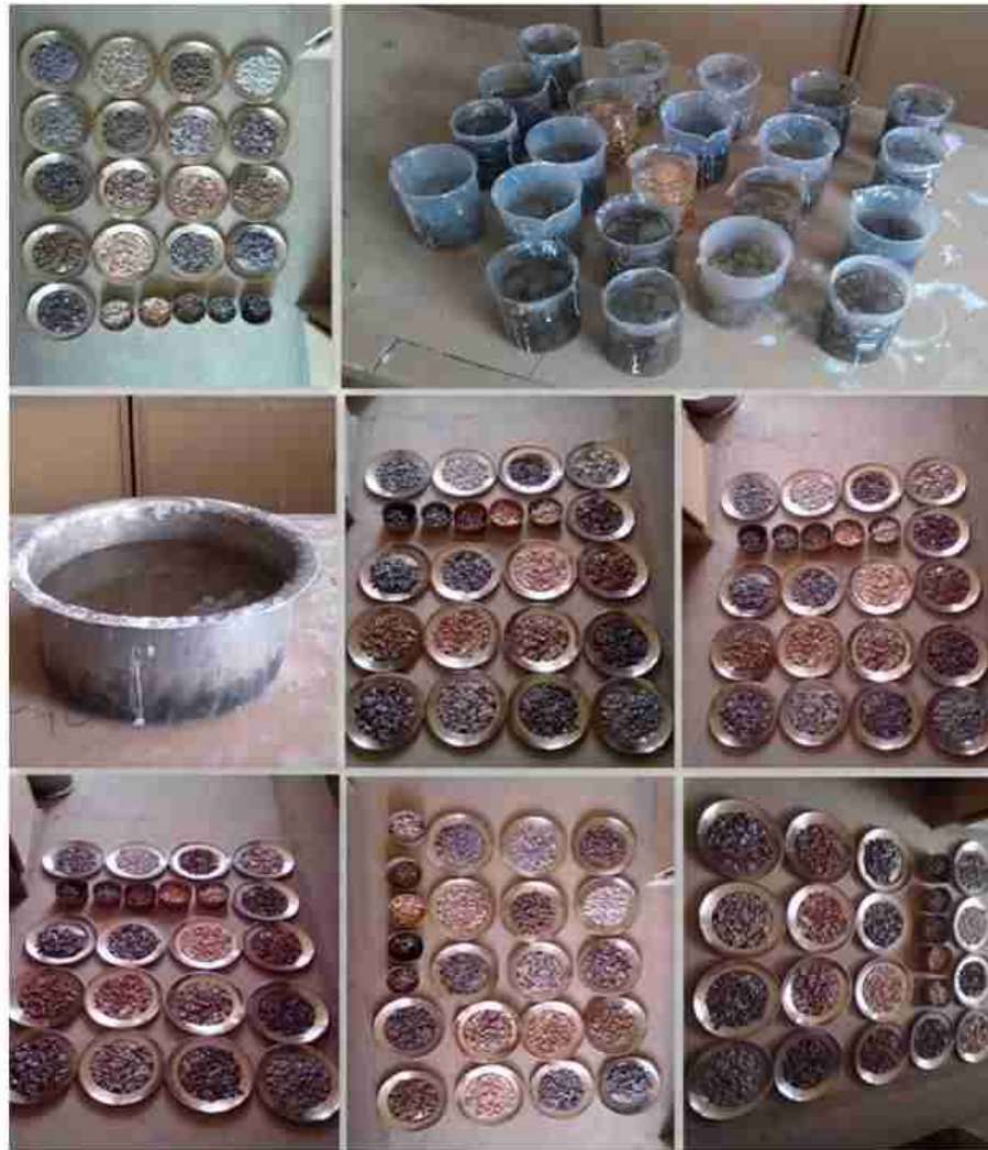
Fig. 3 Samples at different cycles during sodium sulphate soundness test. a) Initial sample before the test, b) Immersion of sample in saturated sodium sulphate, c) Saturated sodium sulphate, d) First cycle, e) Second cycle, f) Third cycle, g) Forth cycle and h) Fifth cycle.
