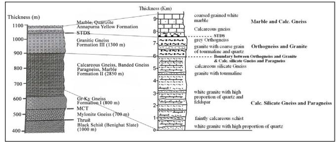
Fig. 6: Correlation of Stratigraphic Columns from the present Study (right) to that of Upreti et al. (2005) in the left
