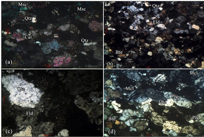
Fig. 5: Mineral contents in (a) Calc. Gneiss (b) (c) Augen gneiss (d) Granitic Gneiss [Qtz: Quartz, Cal: Calcite, Msc: Muscovite, Fld: Feldspar, Bte: Biotite, Mcl: Microcline, Plg: Plagioclase]
