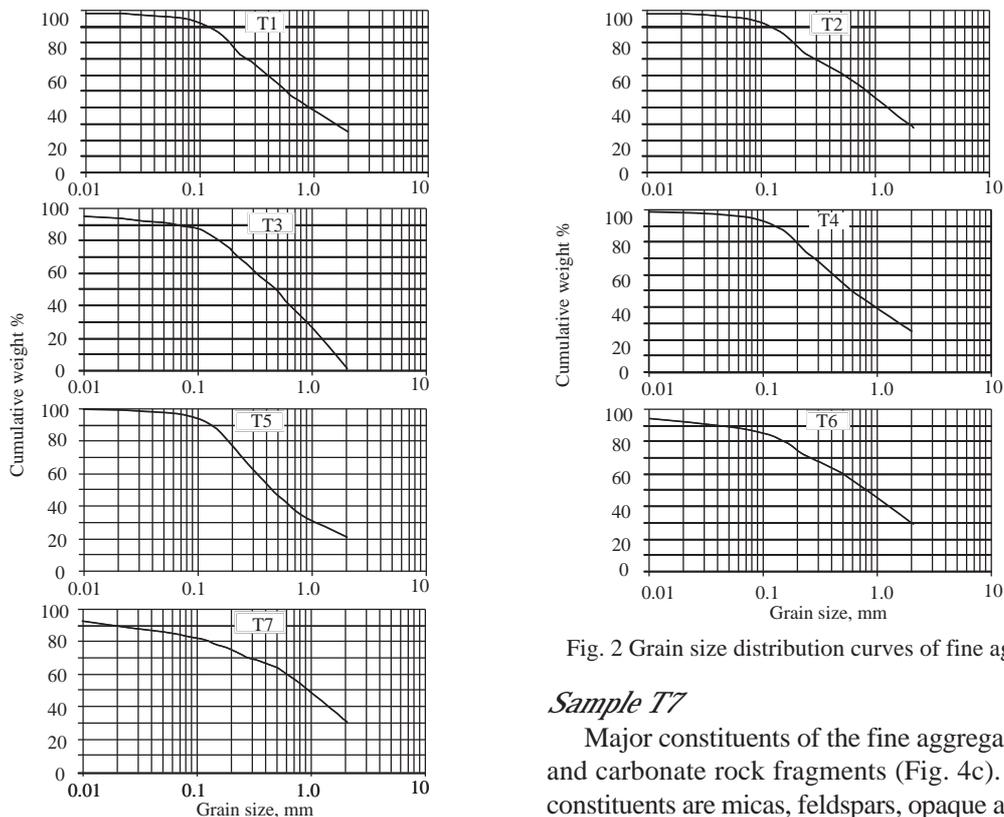
Fig. 2 Grain size distribution curves of fine aggregates.
