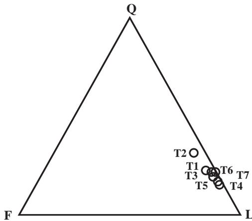
Fig. 3 QFL modes of fine aggregate samples.
