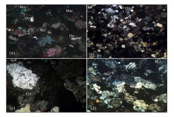
Fig. 5: Mineral contents in (a) Calc. Gneiss (b) (c) Augen gneiss (d) Granitic Gneiss [Qtz: Quartz, Cal: Calcite, Msc: Muscovite, Fld: Feldspar, Bte: Biotite, Mcl: Microclin, Plg, Plagioclase]
