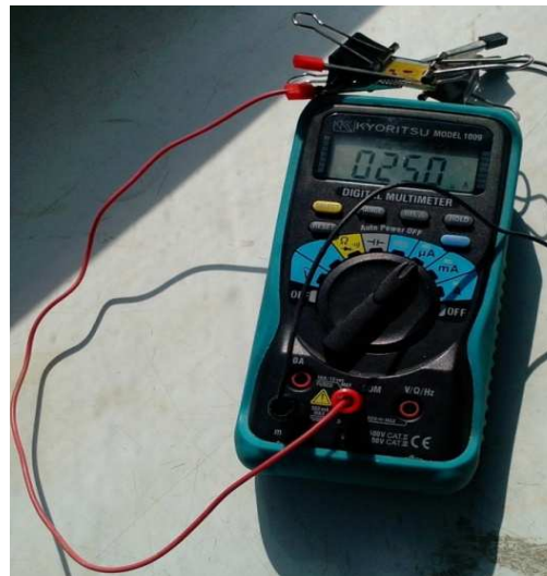
Figure 5: Test of our dye sensitized solar cell (top) in real sun condition. The power of radiation was ca. 930 W. The cell was hold by clamps at the ends and connected to Multimeter. The values on display of multimeter associate voltage (left) and current (right).
