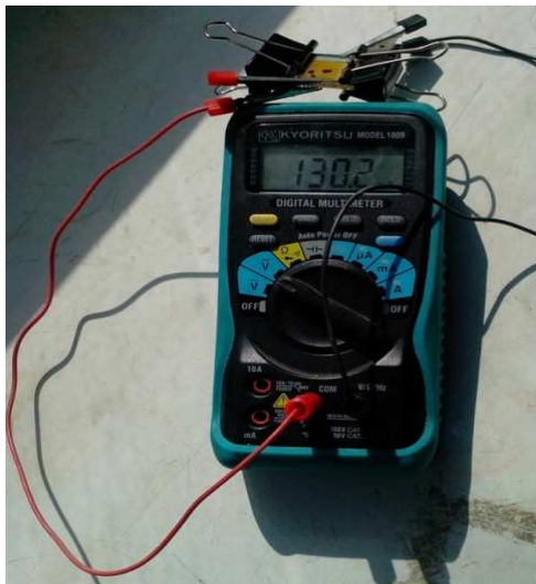
Figure 5: Test of our dye sensitized solar cell (top) in real sun condition. The power of radiation was ca. 930 W. The cell was hold by clamps at the ends and connected to Multimeter. The values on display of multimeter associate voltage (left) and current (right).
