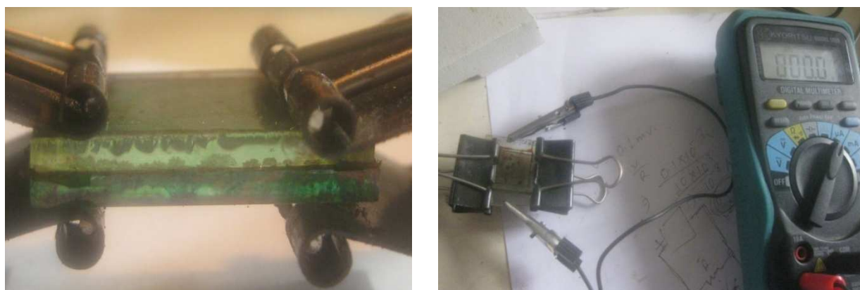
Figure 3: Side view (left) and top view of our proto-type dye sensitized solar cell hold by clamps at the ends. Both the electrodes of the cell shown at right are connected to multimeter for current and voltage measurements.
