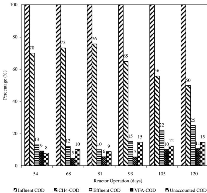
Fig. 4. Carbon (in terms of COD) balance diagram for degradation of glucose bearing SWW.
