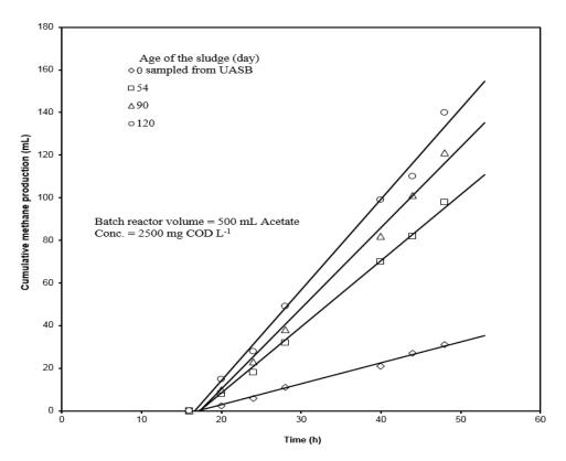
**Fig. 5.** Methane generation profile in the batch tests from the sludge of the different ages sampled from the UASB reactor.
