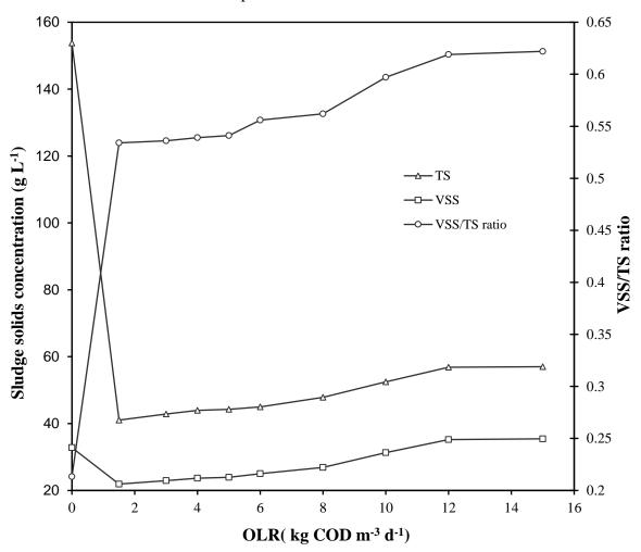
Fig. 2. Variation of sludge solids concentration of the reactor at the end of each OLR.
