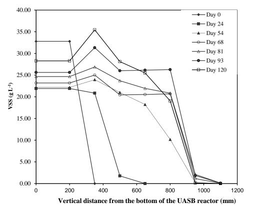
Fig. 3. VSS profile along the height of the reactor on different days.
