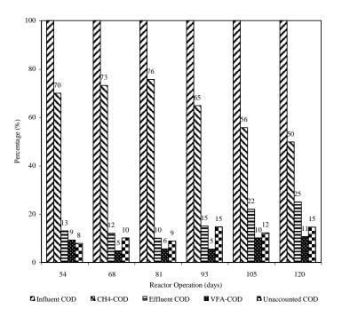
Fig. 4. Carbon (in terms of COD) balance diagram for degradation of glucose bearing SWW.
