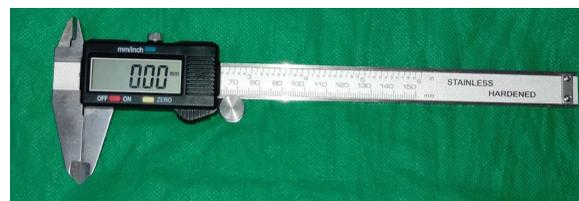
Figure 1: Digital Vernier caliper
