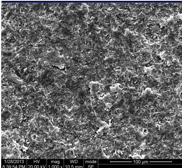
Fig.3 SEM image of ZBR surface.
