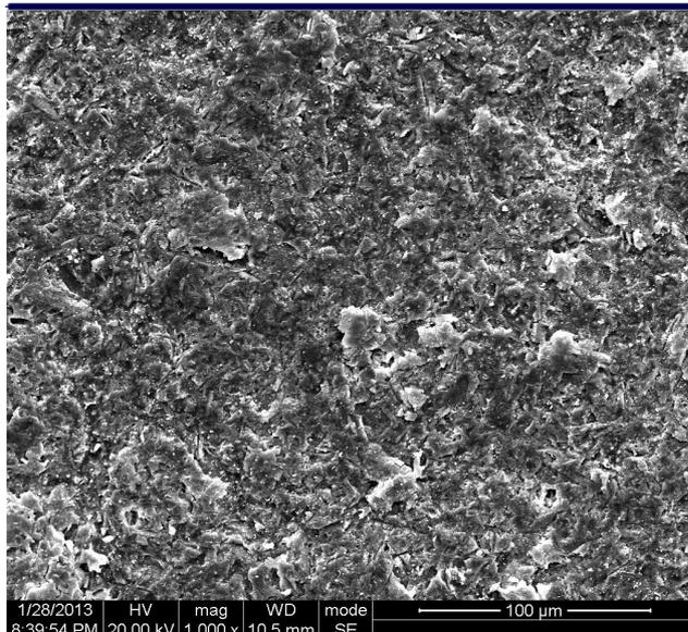
Fig.3 SEM image of ZBR surface.
