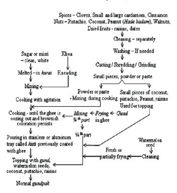
Figure 1. Flow-chart for the traditional production method of normal Gundpak
