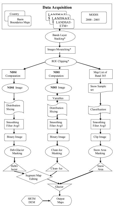
Figure 2: Flow chart of satellite image analysis
