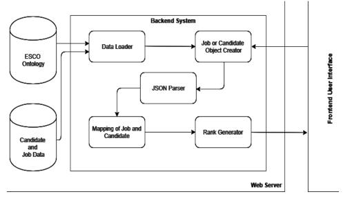
Fig. 3: System architecture
