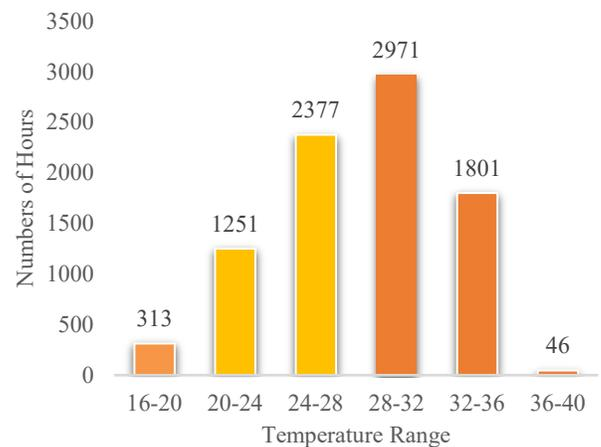
Figure 3: Numbers of Hours in specific temperature range for Biratnagar building
