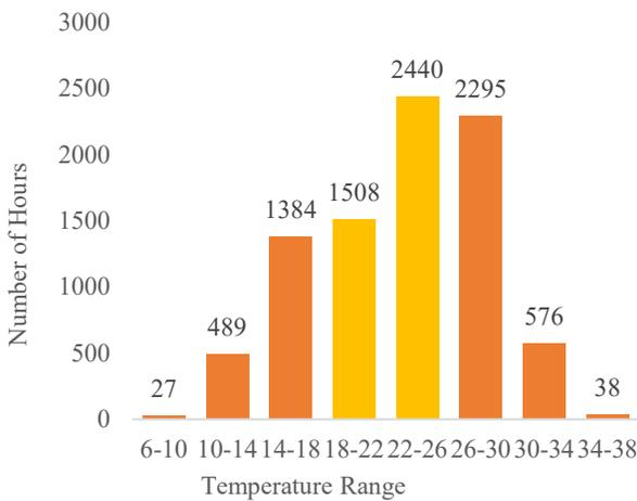
**Figure 4: Number of Hours versus Temperature Range for Dhulikhel Building**
