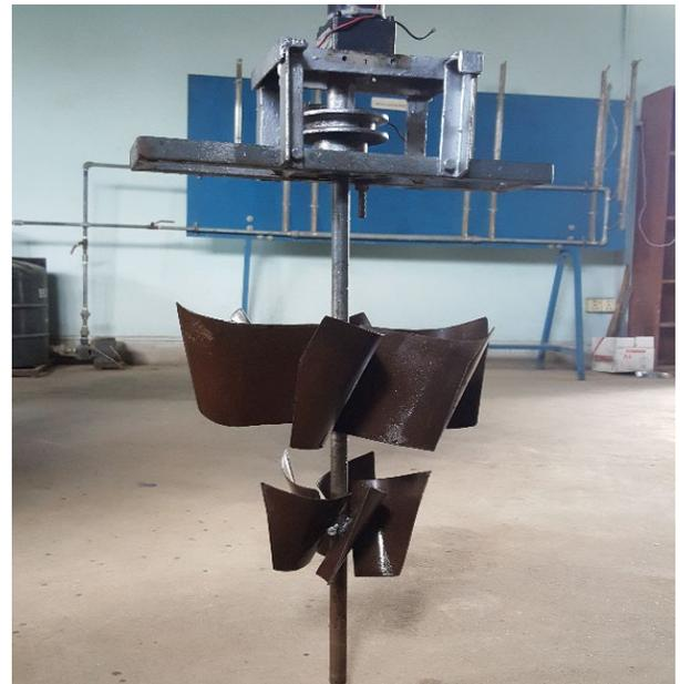
Figure 13: Main runner and booster runner assembly
