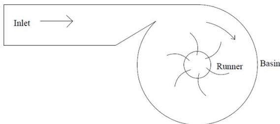
**Figure 1: Working of a GWVPP**
