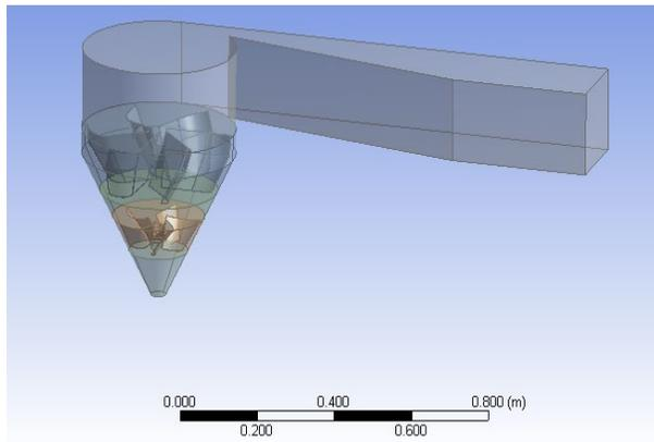
Figure 5: Design modeling of runner and booster
