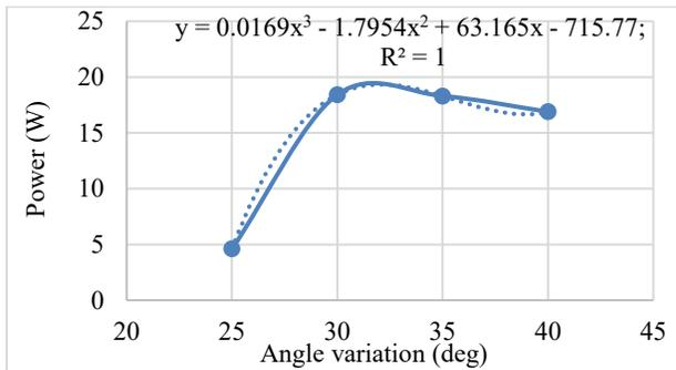
Figure 3: Output power vs blade inclination angle
