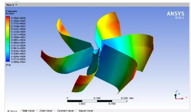
Figure 8: Pressure contour of main runner
