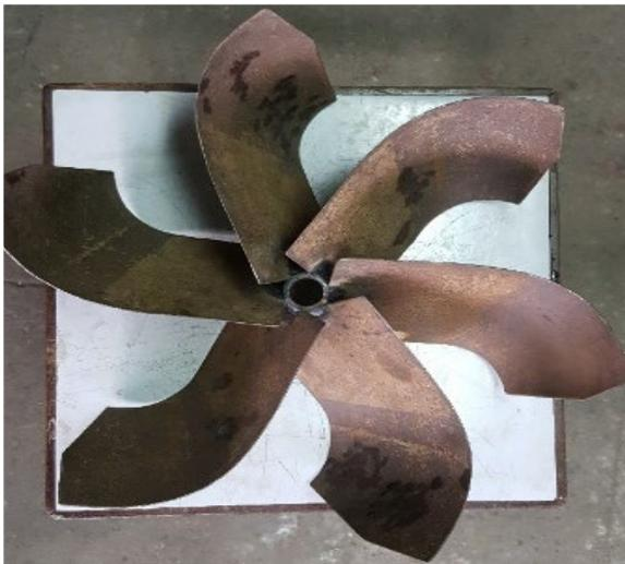
Figure 11: Fabricated main runner
