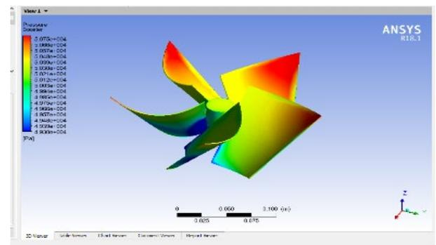
Figure 9: Pressure contour (Booster runner)
