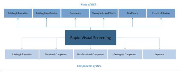
Figure 1: Diagrammatic Representation for Rapid Visual Screening
