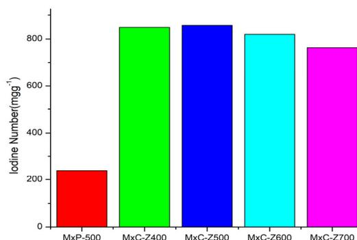
Figure 1: Variation of Iodine number with temperature
