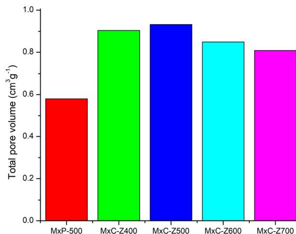
**Figure 5:** Variation of total pore volume with temperature
