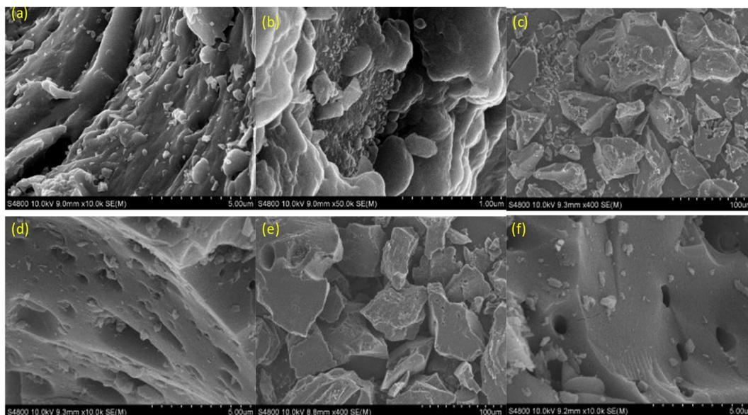
**Figure 7:** Scanning electron microscope (SEM) images of activated carbon materials. (a,b) MxP-500, (c,d) MxC-Z400 and (e,f) MxC-Z500
