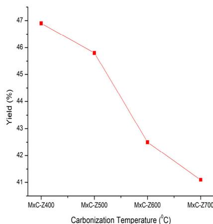
**Figure 6:** The effect of carbonization temperature on yield (%)
