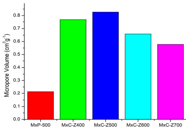
**Figure 4:** Variation of micropore volume with temperature
