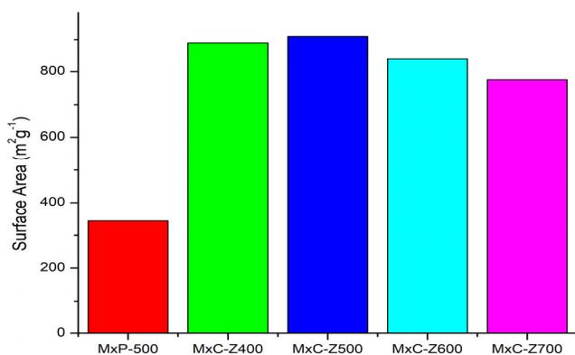
**Figure 3:** Variation of surface area with temperature
