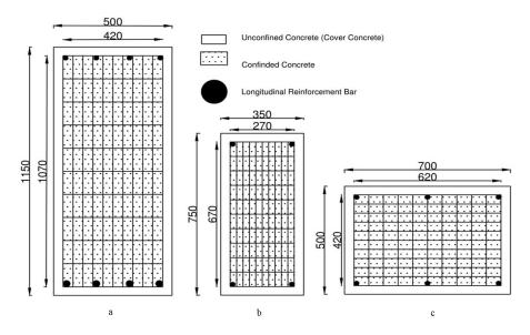
Fig. 2: Fiber section used; a) Arch b) Arch cross beam c) Column
