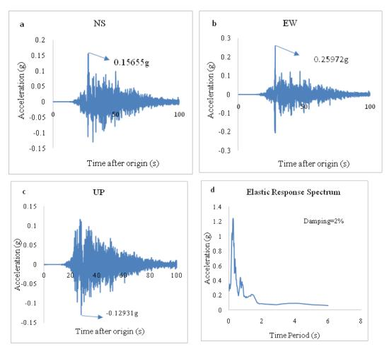
Fig. 3: Ground motion of Gorkha earthquake at KTP station; a) NS b) EW c) Up d) elastic response spectrum
