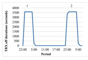
Figure 3: TRX Power off duration for micro BS
