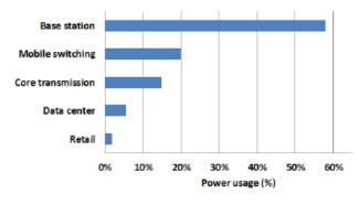
Figure 1: Power Consumption of a Typical Cellular Network
