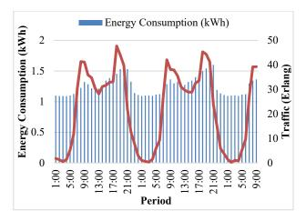
Figure 6: Comparison of energy consumption of macro BS before and after energy after energy saving techniques
