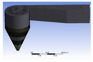
Figure 6: Meshed basin geometry
