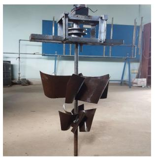
Figure 13: Main runner and booster runner assembly
