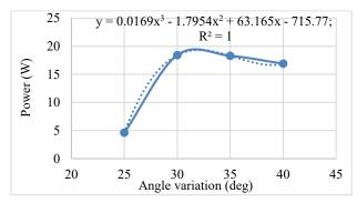
Figure 3: Output power vs blade inclination angle
