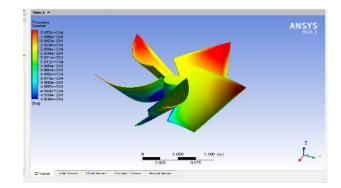
Figure 9: Pressure contour (Booster runner)
