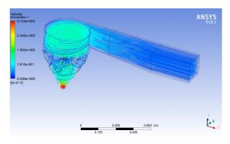
Figure 7: Streamline visualization (Velocity contour)
