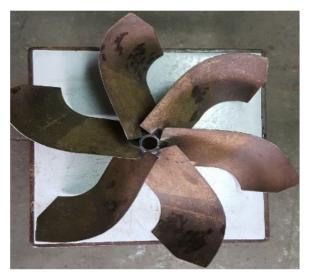
Figure 11: Fabricated main runner
