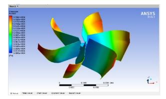
Figure 8: Pressure contour of main runner
