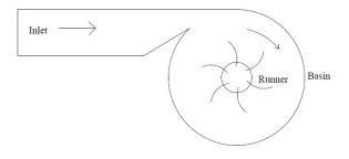
Figure 1: Working of a GWVPP
