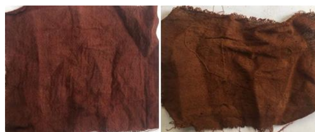
Fig. 8. Photographs showing a comparative colorfastness in cotton cloth dye from E. pulcherrima with K_2Cr_2O_7 and the concentrated black lemon juice, respectively, after washing
