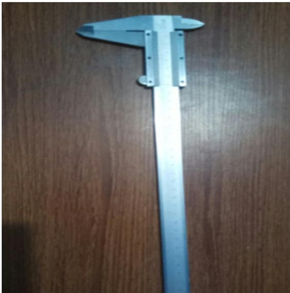
Fig. 1: Sliding Calliper
