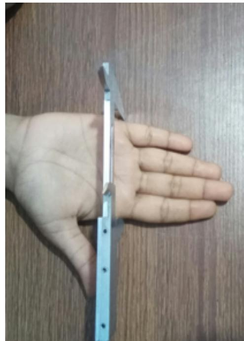
Fig. 3: Measurement of hand breadth
