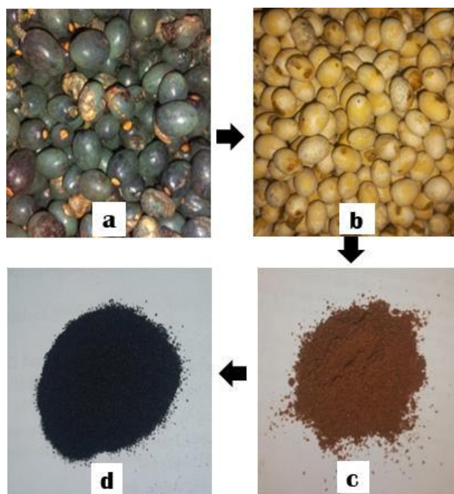
Figure 1: Photographs showing different steps involved during the preparation of activated charcoal from Livistona chinensis seeds: (a) Fruits, (b) Seeds, (c) Seed powder, and (d) Activated charcoal
