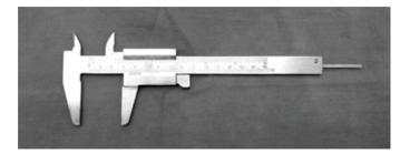
Figure 1: Vernier caliper
