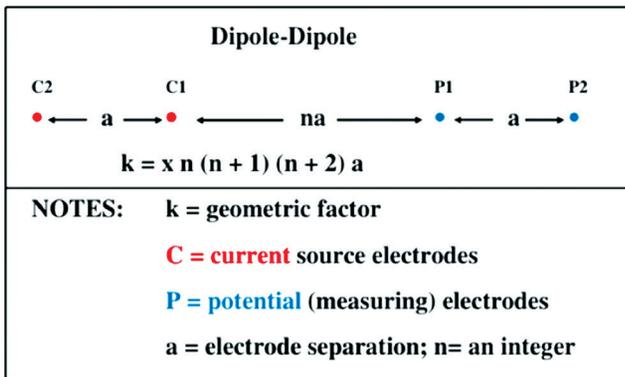
**Fig. 1: Electrical resistivity configuration of dipole-dipole array with the geometric factor (Oldenburg and Jones, 2007).**
