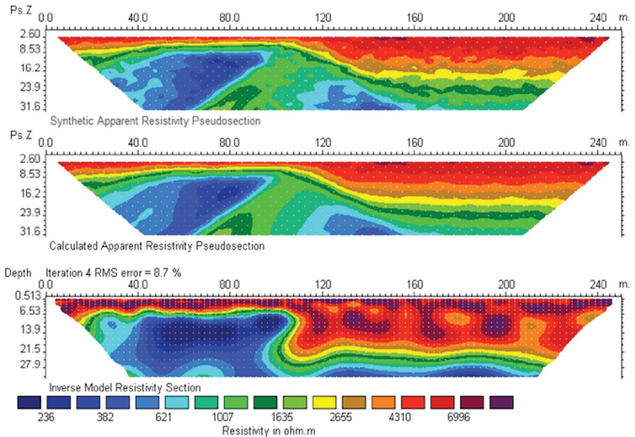
Fig. 9: Inverse resistivity sections for the collapse mass II at 10% noise level.
