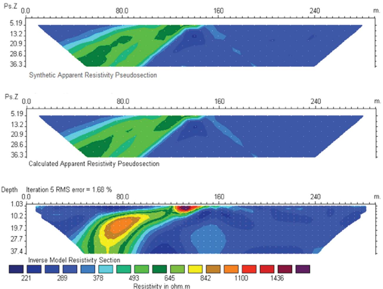
Fig. 3: Inverse resistivity sections for the collapse mass I at 2% noise level.
