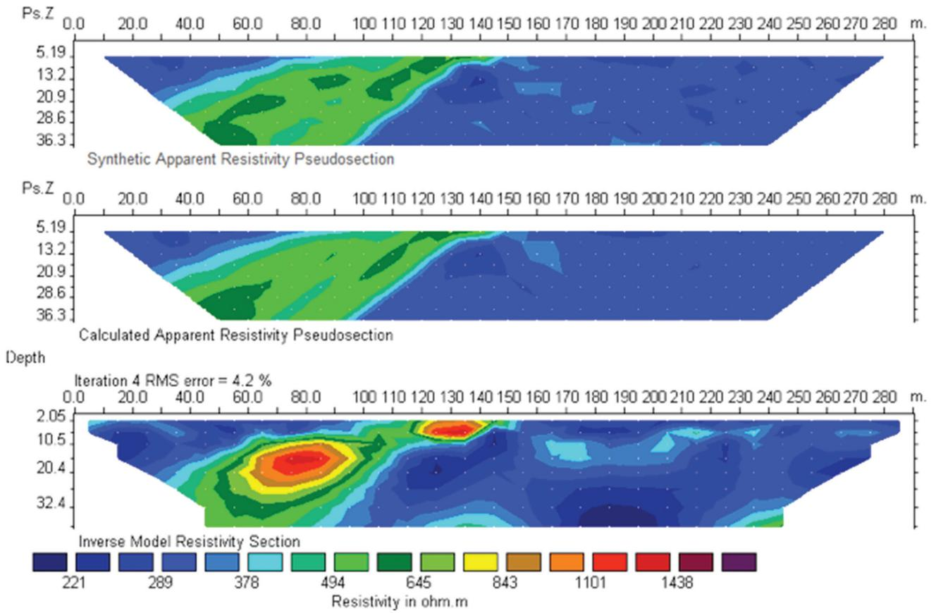
Fig. 4: Inverse resistivity sections for the collapse mass I at 5% noise level.
