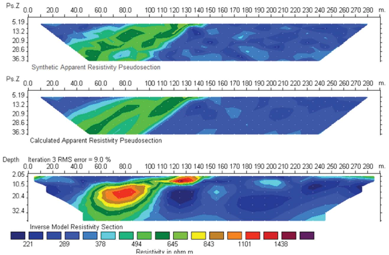
Fig. 5: Inverse resistivity sections for the collapse mass I at 10% noise level.
