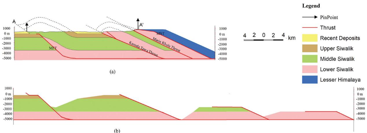
**Fig. 5: (a) Balanced cross-section and (b) Restored cross section along A-A' in Fig. 3.**
