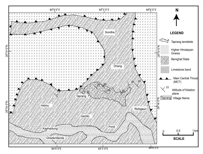
Fig. 2: Generalized Geological Map of the Landslide Area (modified from Regmi et al., 2017).
