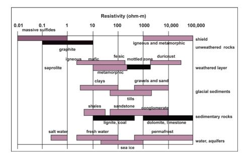
Fig. 8: Common resistivity values of earth materials (after Palacky, 1980).
