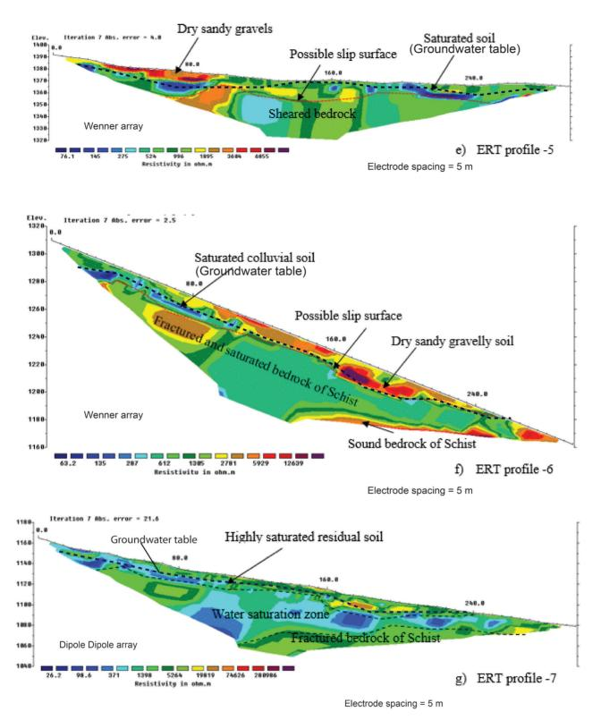
Fig. 7: Electrical resistivity tomography results (a) Profile-1 across the landslide at crown (b) Profile-2 along the landslide movement at crown (c) Pofile-3, across the landslide at body part (d) Profile-4, along the landslide at body part (e) Profile-5, along the landslide at body part (f) Profile-6, along the landslide at left flank of the toe part (g) Profile-7, along the left flank of landslide at toe part.
