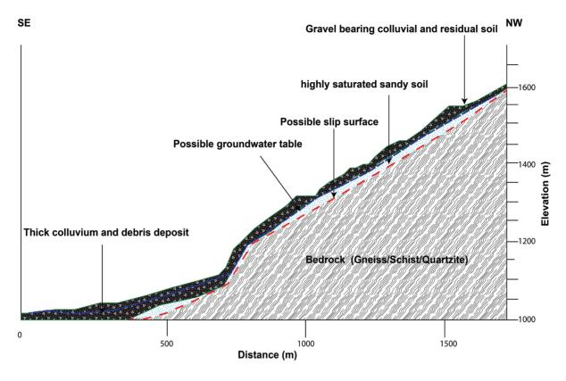
Fig. 9: Longitudinal-section of the Taprang landslide showing different lithological layer and slip surface.
