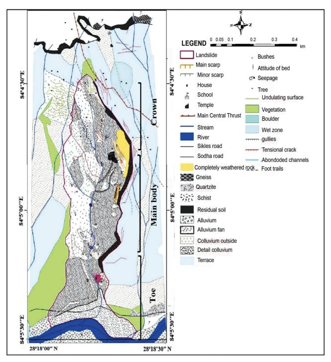
Fig. 3: Morphological map of the Taprang landslide.
