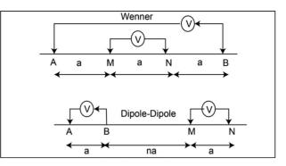
Fig. 5: General electrodes configuration of ERT survey (Griffiths and Turnbull 1985; Loke and Barker 1996).
