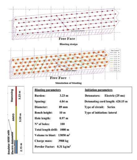
Fig. 3: Blasting data and Simulation of blasting.
