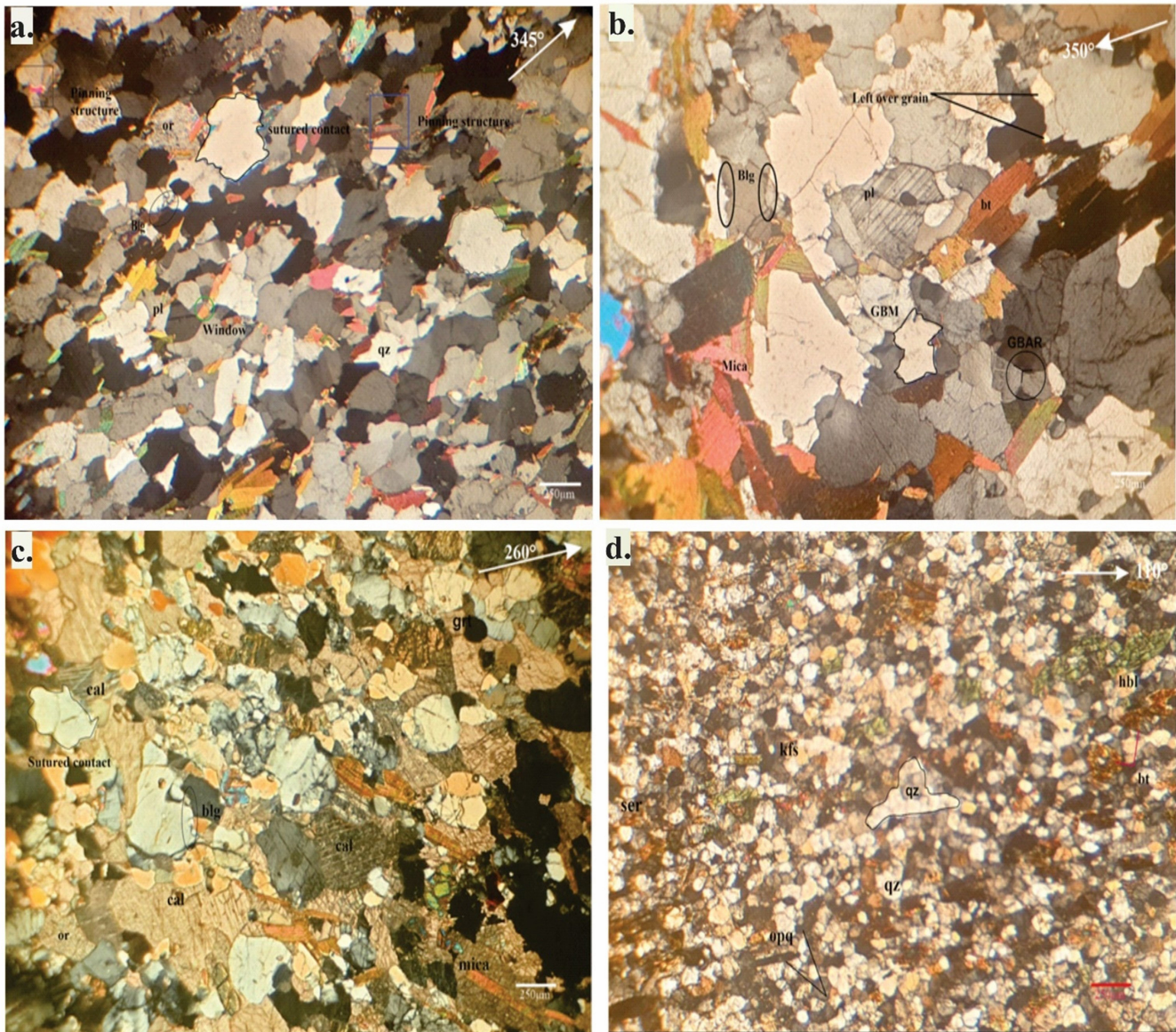
Fig.7: Photomicrograph of samples under cross polarizing light: a) Showing sutured, pinning window structures observed near Sisneri area under cross polarizing light (27°49'3.54"N, 85°12'40.91"E), b) granitic gneiss showing both dynamic and static recrystallization under cross polarizing light (27°48'51.13"N, 85°12'42.89"E), c) calc-silicate gneiss showing Blg, calcite observed near Ranipauwa park under cross polarizing light (27°49'43.94"N, 85°14'10.82"E), and d) metasandstone from Tistung Formation observed near Jalukelp showing the irregular boundary of quartz crystals Under cross polarizing light (27°47'29.80"N, 85°16'6.33"E).
