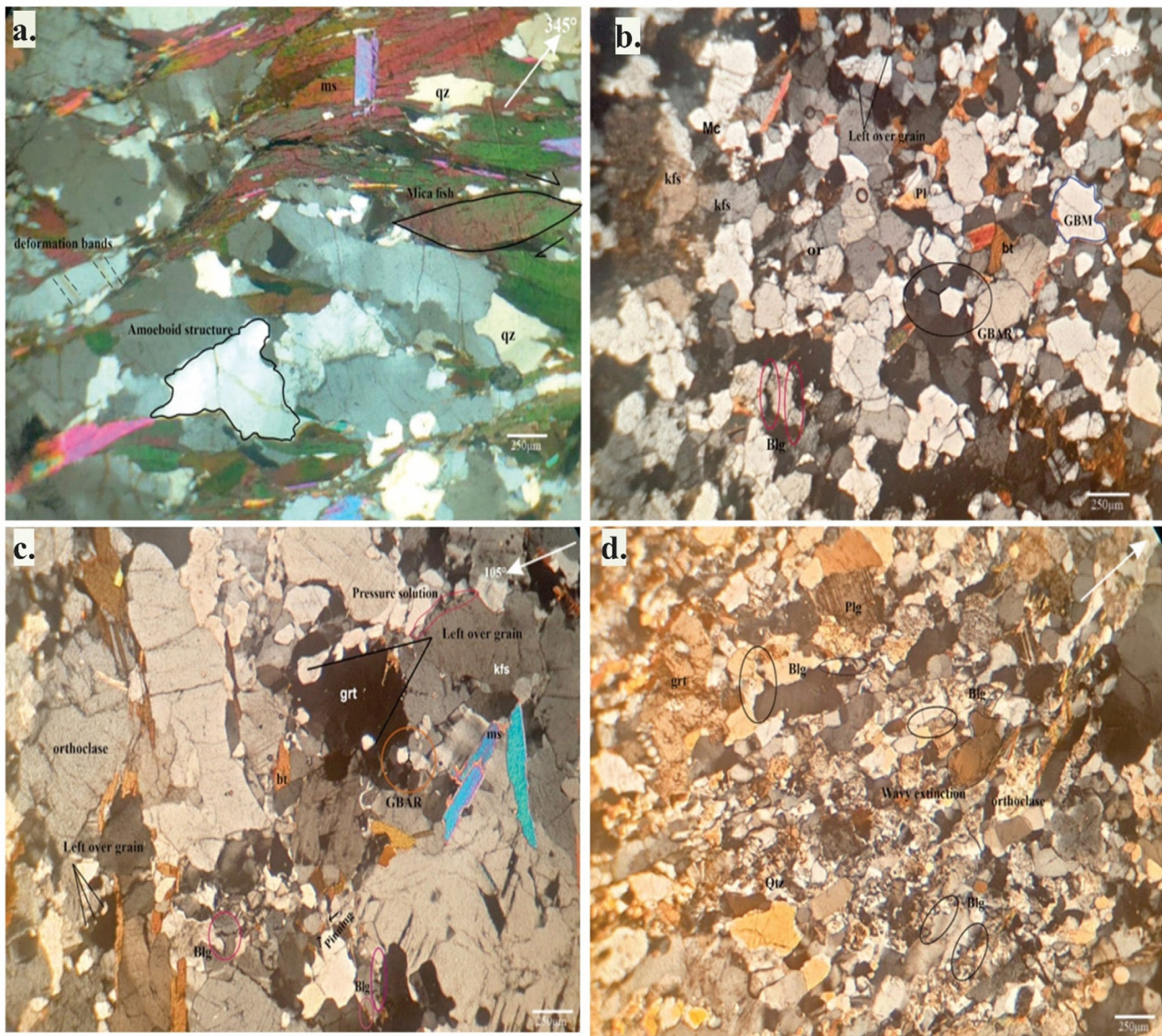
Fig. 6: Photomicrograph of samples under cross polarizing light; a) Granite showing sutured contact and mica fish observed in 10x magnification (27°50'16.79"N, 85°10'15.59"E), b) showing both dynamic and static recrystallization observed in 10x magnification (27°50'16.17"N, 85°10'16.52"E), c) showing dynamic recrystallization and triple junction observed in 10x magnification (27°50'4.35"N, 85°11'35.11"E), and d) granitic gneiss showing big, wavy extinction observed in 10x magnification (27°49'22.77"N, 85°12'36.31"E).
