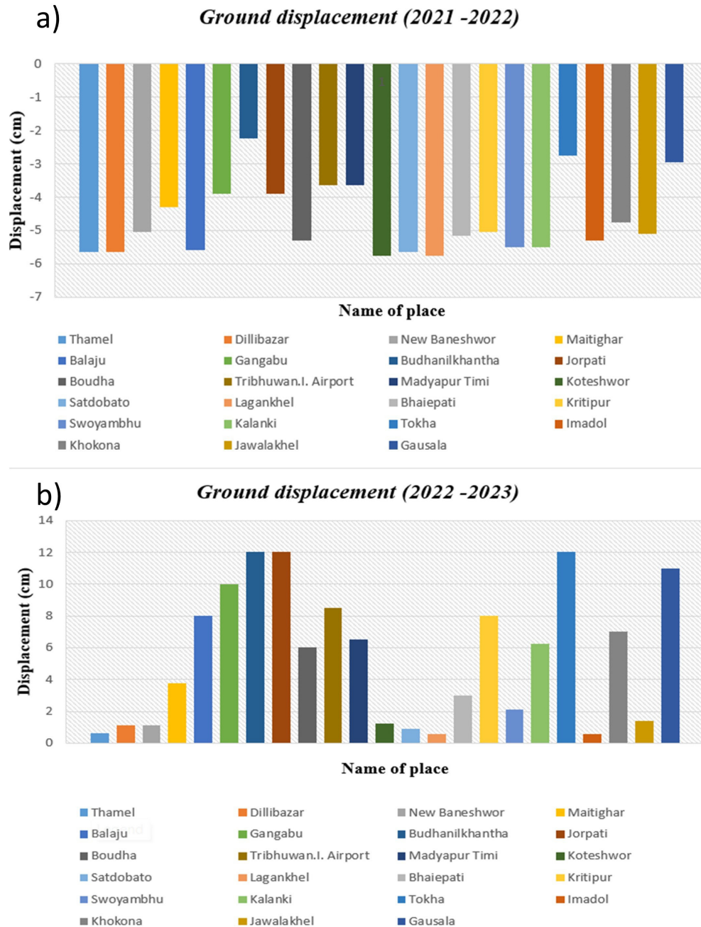
Fig.10: Ground displacement for (2021 - 2022) left and (2022-2023) right along with the name of place indicated with different colors.
