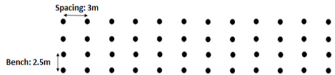
Fig. 7: Drilling plan for the calculated holes.
