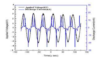
**FIGURE 2.** Current voltage graph at argon flow rate(Q) = 3 L/min at an applied voltage of 3.5 kV
