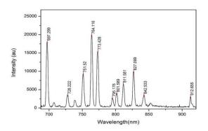
**FIGURE 3**. Spectra of the discharge at frequency 20 kHz and an applied voltage of 3.5 kV(Q=3 L/min)
