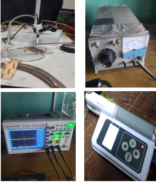
FIGURE 2: (a) Plasma treating on Seed, (b) Power supply, (c) Digital oscilloscope, (d) Chlorofillmeter
