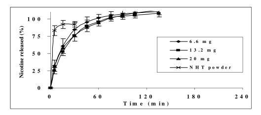
Fig. 7 Release (%) profile of nicotine from K4MP powder blends, each containing 4 mg nicotine base (as hydrogen tartrate). The amount of K4MP in the powder mixes indicated, 6.6, 13.2, & 20 mg, is the same as in lyophilisates prepared from 1, 2 & 3% K4MP solutions respectively. 11.4 mg nicotine hydrogen tartrate (NHT powder) equivalent to 4 mg nicotine base, was used as a control. Each data point is mean  $\pm$ s.d.of three experiments.
