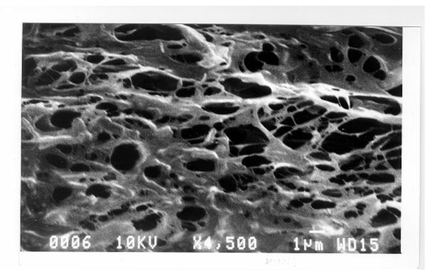
Fig. 8 SEM picture of a lyophilisate prepared from 2% K4MP solution containing NHT.
