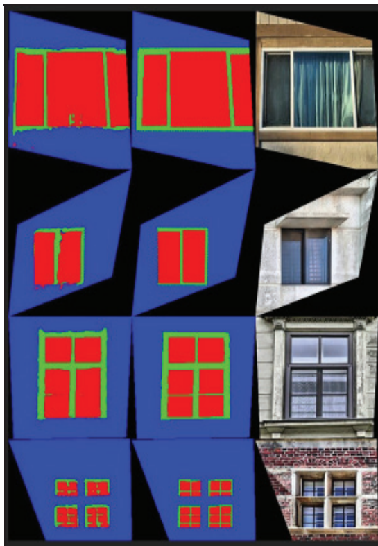
Figure 8: Semantic segmentation results (rectified)
