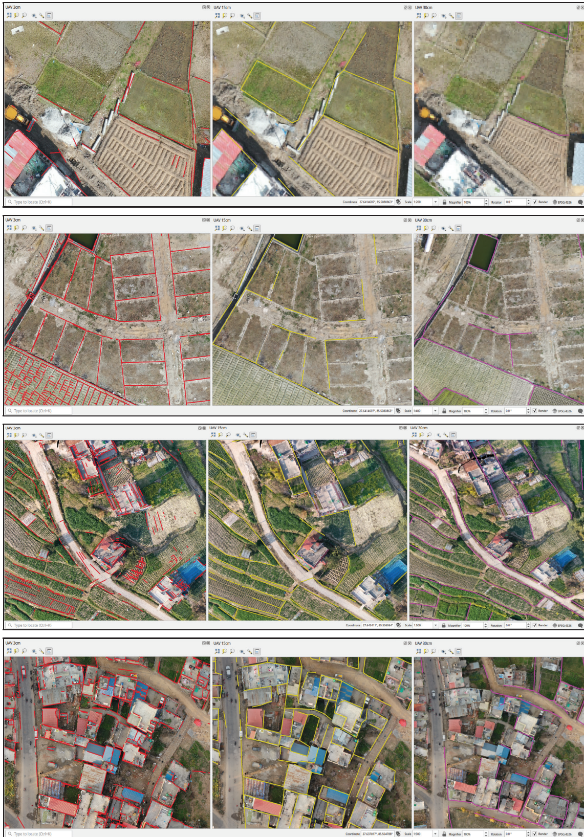
Figure 2. Predicted boundary polylines (colored overlays) generated by the classifier, shown overlaid on UAV orthophotos at 3 cm, 15 cm, and 30 cm resolutions
