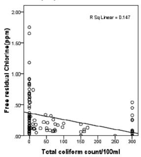
Fig. 2. Relation between free residual chlorine and total Coliform counts
