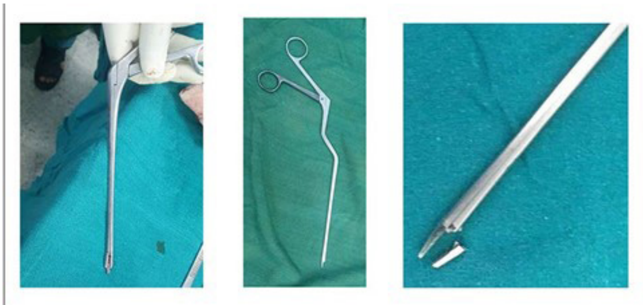
Fig. 3: Bigger size pituitary rongeur which was used to remove the metallic foreign body and 2mm size pituitary rongeur whose tip was broken
