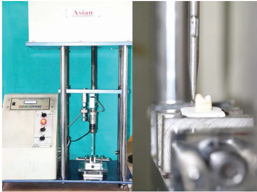
Fig 7: Debonding done by Universal Testing Machine (UTM)
