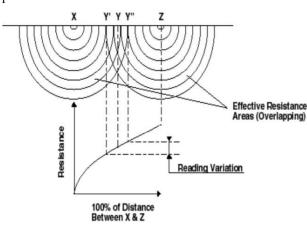
Figure 4: Schematic diagram for working of auxiliary rod. [Adapted from 15, 16]
