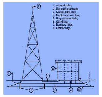
Figure 1: Components of lightning protection system on a tower as per IEC 62305. [Adapted from 9]
