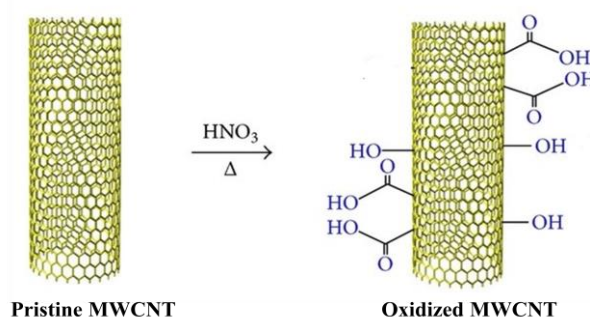
Scheme 1: Schematic representation of formation of oxidized MWCNTs.
