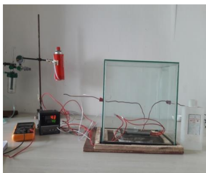
Figure 2: Experimental set up for ethanol sensor.
