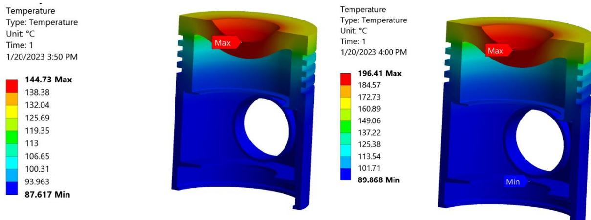
Figure 11: Temperature distribution due to  $Q_1$ Figure 9: Temperature distribution due to  $Q_2$
