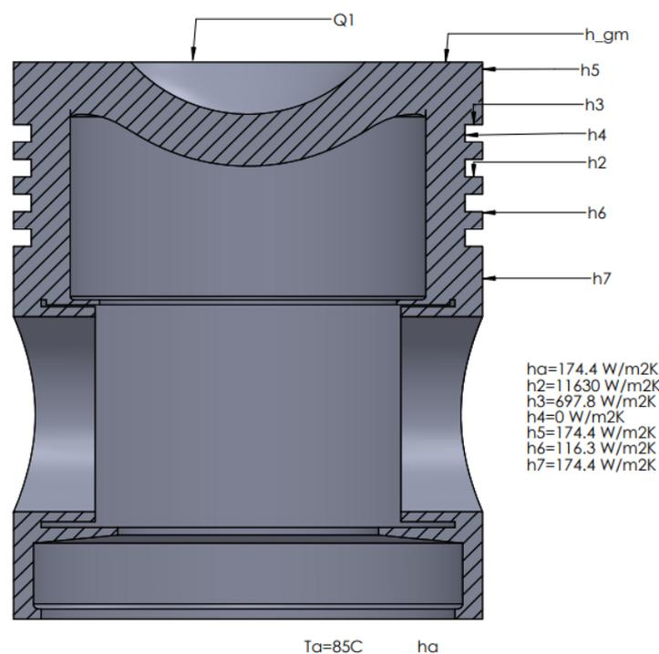
Figure 6: Boundary condition of an aluminum alloy internal combustion engine piston
