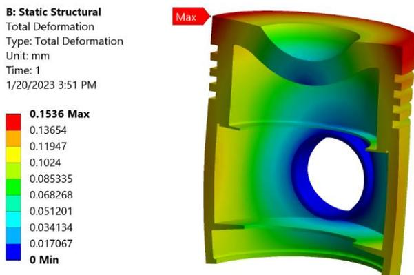
Figure 9: Deformation due to  $Q_1$
