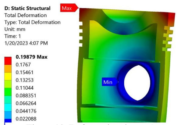
Figure 10: Deformation due to  $Q_2$
