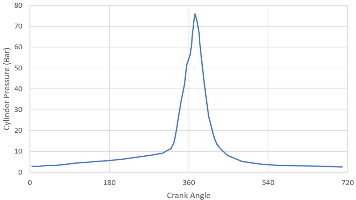
Figure 3: Variations of in-cylinder pressure in diesel engine with crank angle (Muhammad Usman Kaisan, 2021), (Torregrosa, 2007)
