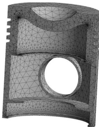
Figure 5: Mesh used in the simulation
