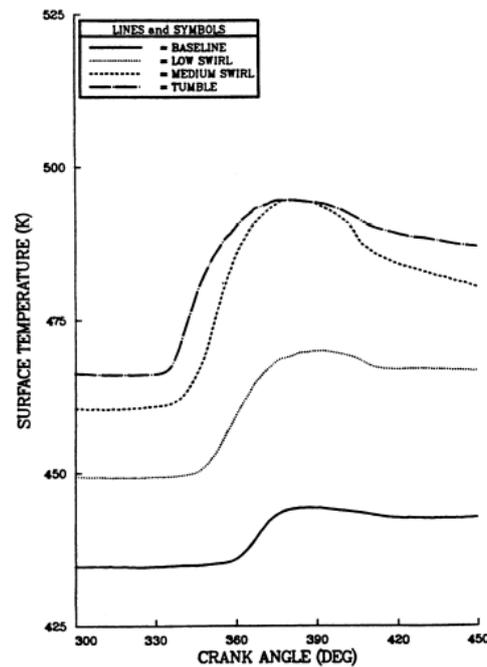
Figure 2 : Effects of flow configuration on surface temperature (Alkidias, 1990)
