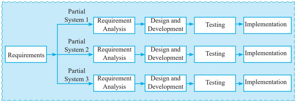
**Figure 1: Block Diagram of Incremental Model**
