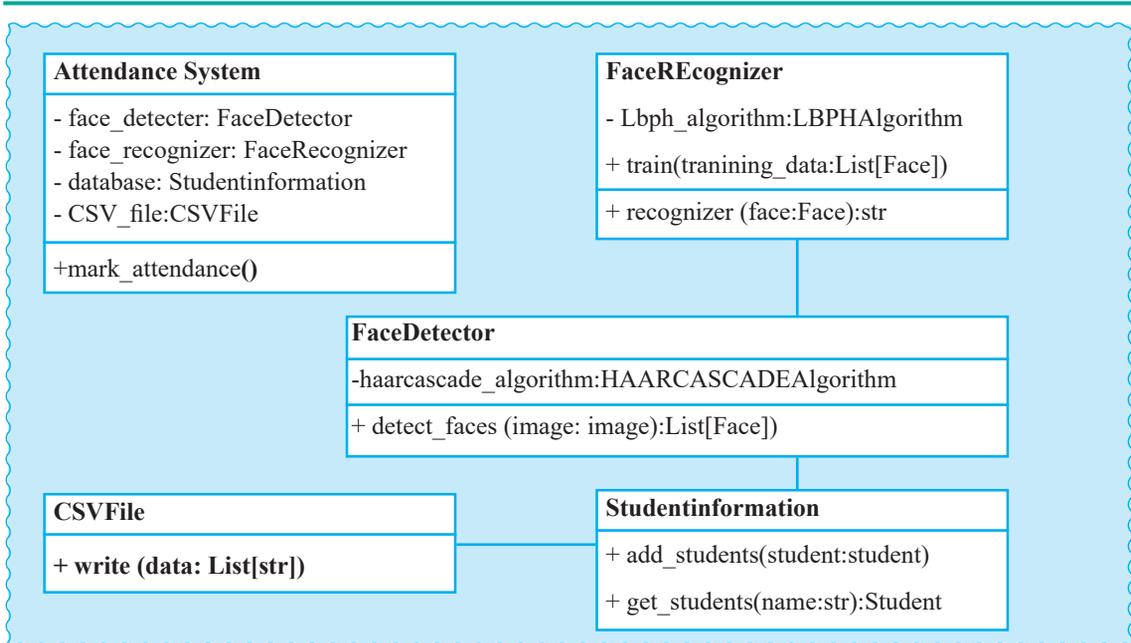
**Figure 3: Class Diagram of an Automated Attendance System**
