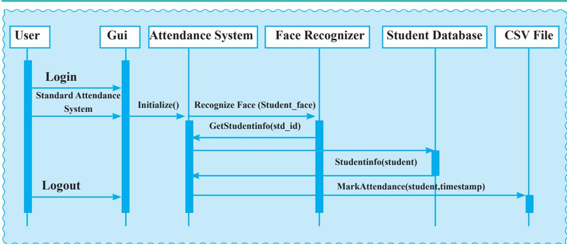
Figure 5: Sequence Diagram of an Automated Attendance System
