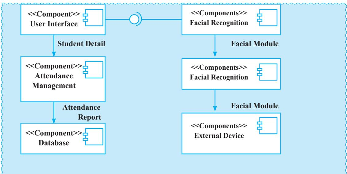
Figure 6: Component Diagram of an Attendance System
