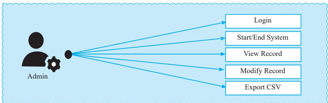
*Figure 2: Use-Case Diagram of An Automated Attendance System*
