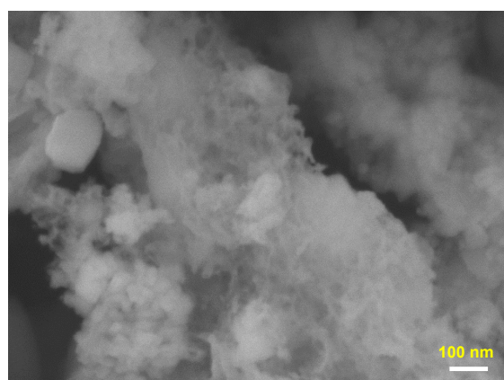
Fig. 5. SEM image of synthesized Rud-AgNPs
