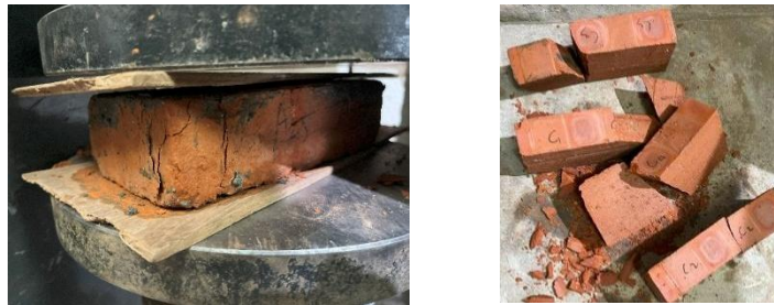
Figure 2. Crushing Strength test of brick samples
