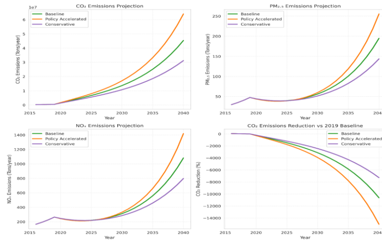
Figure 3 (a-c). Projected emissions of CO 2 , PM 2.5 , and NO x under the three scenarios. (d) Percentage reduction in CO 2 emissions compared to the 2019 baseline, highlighting the combined effect of fleet electrification and grid decarbonization.
