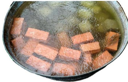
Figure 3. Curing of brick samples (24-hour water immersion)
