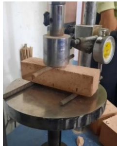
Figure 9. Cuboid specimen under axial loading in UTM
