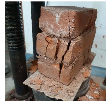
Figure 6. Vertical cracks on the masonry prism
