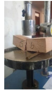
Figure 10. Failed cuboid after testing
