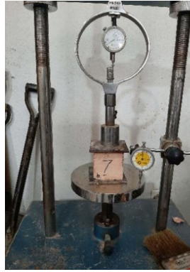
Figure 2. Cube specimen under axial loading
