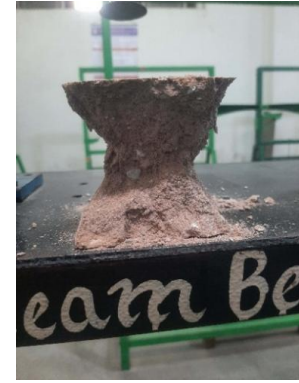
Figure 3. Failed cube after testing
